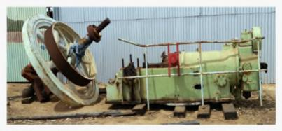
manufactured by the Crossley Brothers of Manchester England between 1923 and 1930 with Model - HH14 - the more powerful type HH - with a slightly larger cylinder bore and the same piston stroke compared to the HD / HDE of the same size, this results in increased power output.
