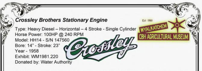
This 1958 Crossley Stationary Engine was used to drive a water pump at Minnivale Pumping Station. Installed when reticulated water was fed to the Town of Wyalkatchem from the Kalgoorlie pipeline via Cunderdin.
